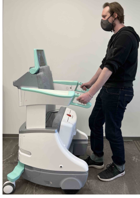
Fig. 1. Example use case for the algorithm presented in this paper. A user walks with an assistive mobility robot. A camera is mounted on the robot that is intended to capture the head of the user.
